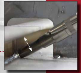
Maintaining proper weld gun angles
